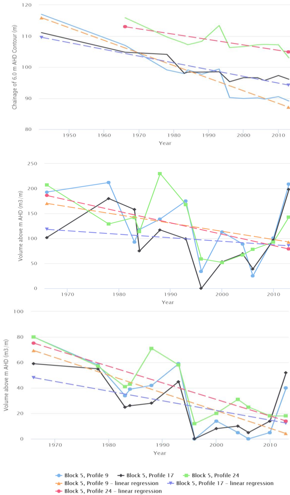
Figure 6: Toolbox results for three profiles at Wooli. From top to bottom: escarpment monitoring contour (6 m AHD), sub-aerial beach volume (above 0 m AHD) and dune volume (above 2.5 m AHD).
